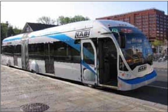
Bus Rapid Transit (BRT) vehicles are alternatives to light rail vehicles with fixed rails. BRT vehicles can operate on existing roadways with little roadway modification.
